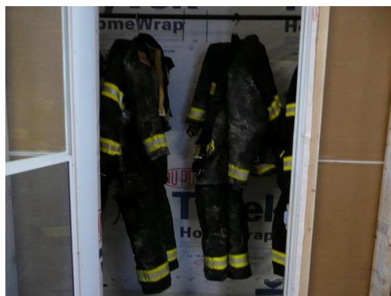
The enclosure was intended to represent the volume of a typical 6-seat apparatus cabin. Air sampling was conducted for VOCs (n = 12 for each group) and HCN (n = 12 for each group) over a 15-min period, intended to represent the driving time to and from the station.
