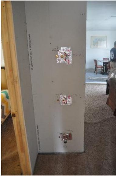
Heat flux (the speed of thermal energy transfer) measurements were made using a 1-in nominal diameter water-cooled Schmidt-Boelter heat flux gauge. The gauges measured the combined radiative and
