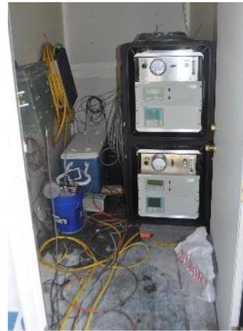
Pressure measurements were made in every room at 3 elevations; 1 ft, 4 ft, and 7 ft above the floor. The pressure recorded was a differential pressure between the inside and outside of the structure.
