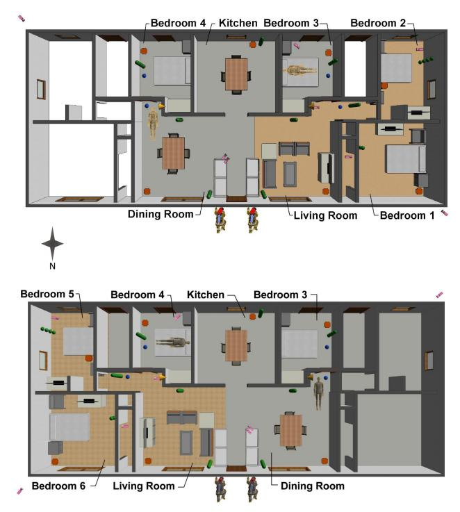
*Figure 4. Layout of burn structure showing false wall set up for the (top) right side experiment layout and (bottom) left side experiment layout.*
