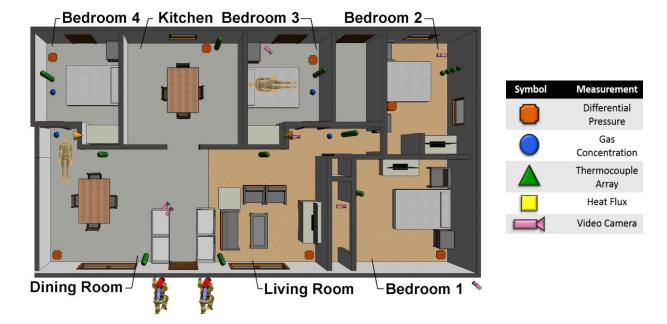
Figure 10. Measurement layout in the right side configuration
