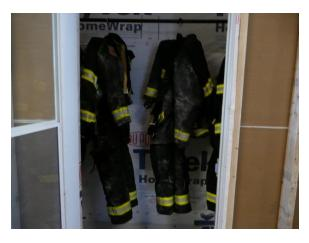
The enclosure was intended to represent the volume of a typical 6-seat apparatus cabin. Air sampling was conducted for VOCs (n = 12 for each group) and HCN (n = 12 for each group) over a 15-min period, intended to represent the driving time to and from the station.
