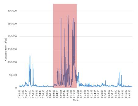
Figure 15. Particle number concentrations (for particles 0.01 to > 1  $\mu$ m) measured at the fire ground (south of Engine 1) on 6/30/2015. Red shading represents the period between structure fire ignition and suppression/start of overhaul.
