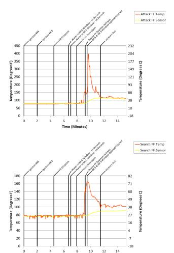
Figure 19. Helmet mounted temperature measurements collected from (top) nozzle firefighter on the attack team and (bottom) lead search team member (06/14/2015). The orange line is the gas temperature in the vicinity of the firefighter, while the yellow line is the internal sensor temperature (can be ignored for now).
