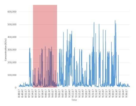
Figure 14. Particle number concentration (for particles 0.01 to > 1  $\mu$ m) measured at the fire ground (south of Engine 1) on 6/27/2015. Red shading represents the period between structure fire ignition and suppression/start of overhaul.
