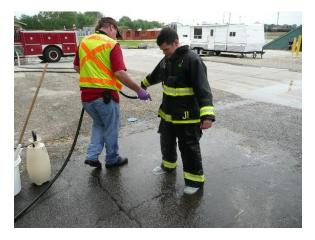
Turnout gear sampling: surface wipe sampling
