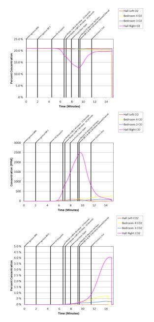
Figure 18. Gas concentrations from closed bedrooms and hallway locations, including (top) oxygen, (middle) carbon monoxide and (bottom) carbon dioxide (06/14/2015).
