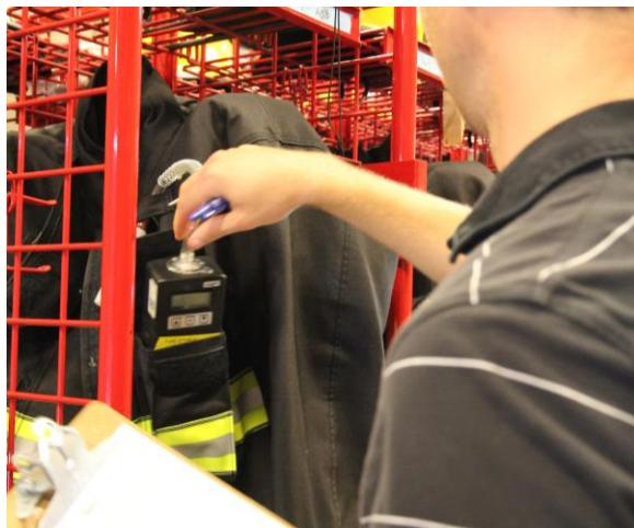
hydrocarbons (e.g., benzene, toluene, xylenes). The sampling pumps were started before firefighting commenced and stopped when the firefighters returned to the bay for doffing of their gear. Air concentrations were determined based on the time that the sampling pumps operated during the fire response. A total of 144 personal air samples for each class of compounds was collected.
