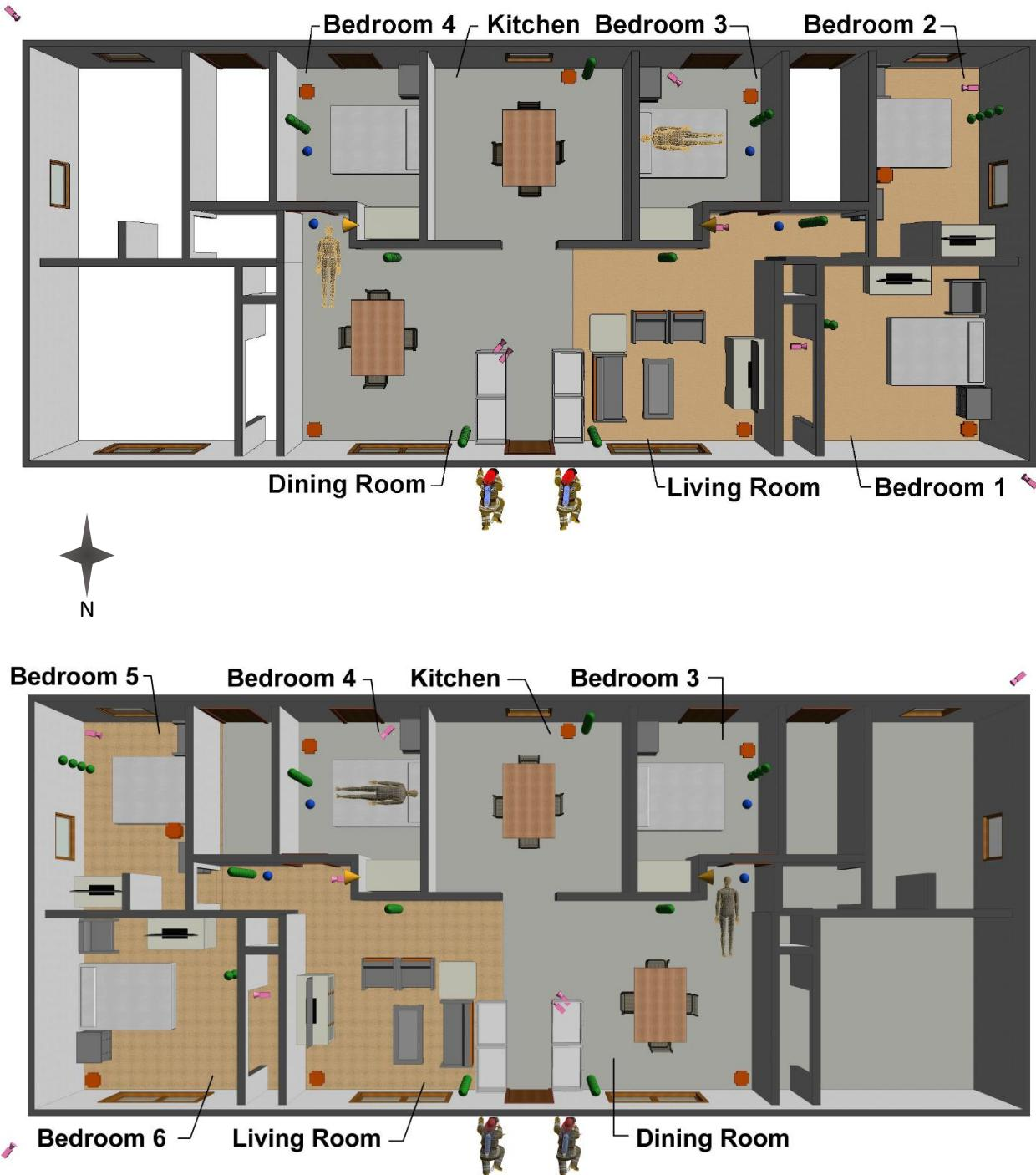
*Figure 4. Layout of burn structure showing false wall set up for the (top) right side experiment layout and (bottom) left side experiment layout.*
