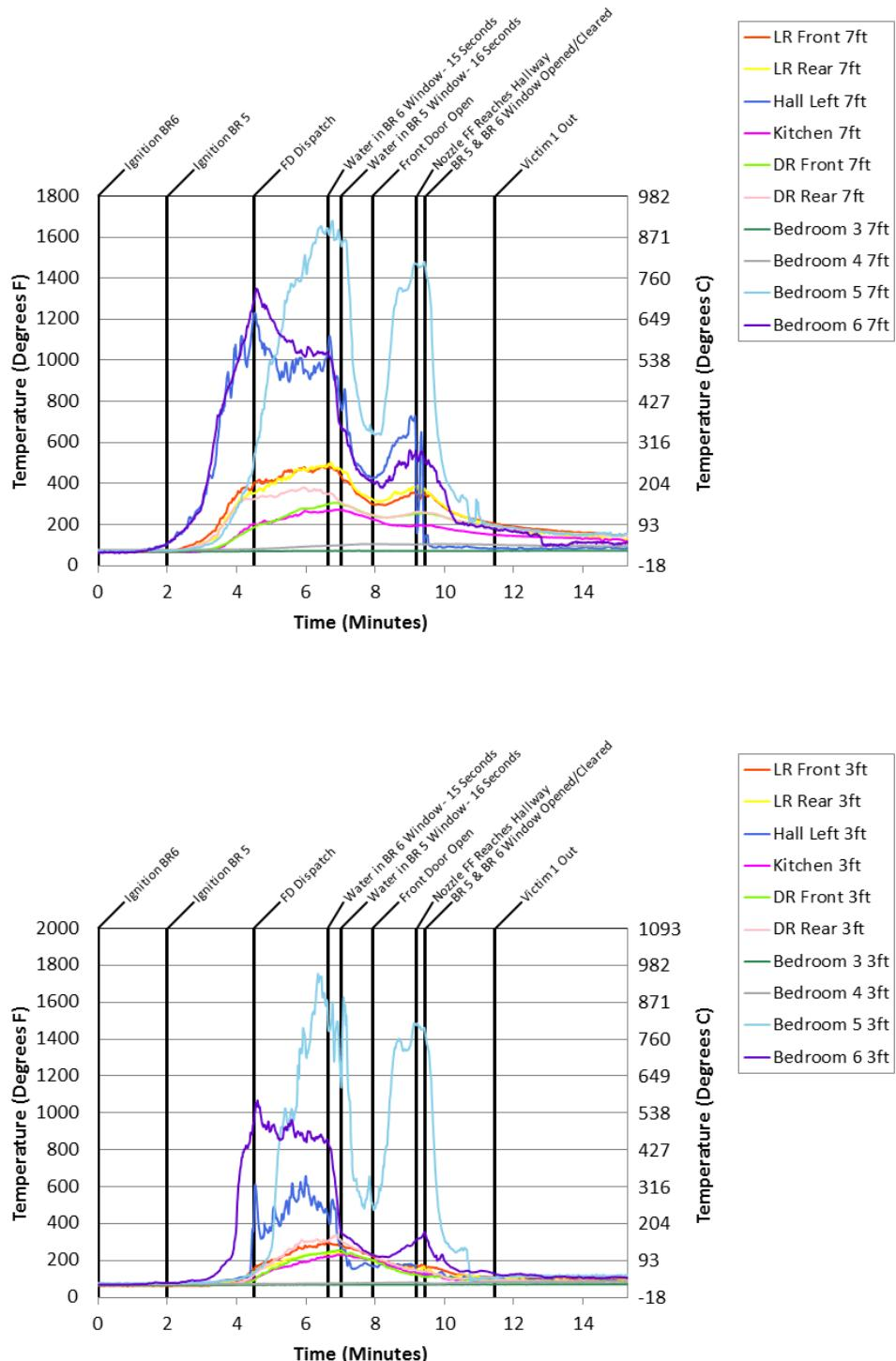
*Figure 16. Building gas temperatures at each of the measurement locations of the structure (LR = Living Room, DR = Dining Room) for an example transitional attack scenario (06/14/2015).*
